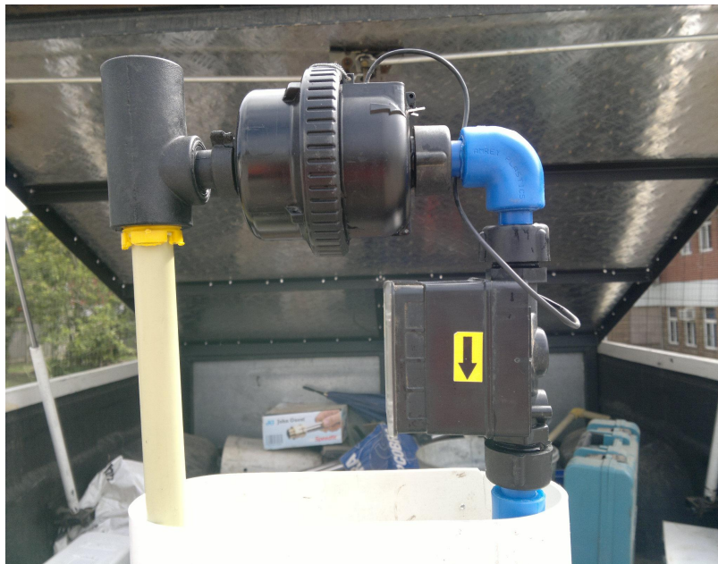
A flow limiter connected to the pulse output of a water meter
